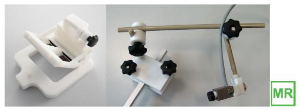
The head-coil mount fits the camera to the head-coil (specific to particular head-coil and scanner, example on the left). Alternatively a "universal" camera mount is available (picture on right).
